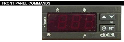
SET: To display target set point; in programming mode it selects a parameter or confirms an
